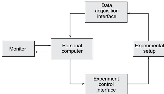
**Fig. 2.1** Block diagram of a personal computer-controlled experiment
