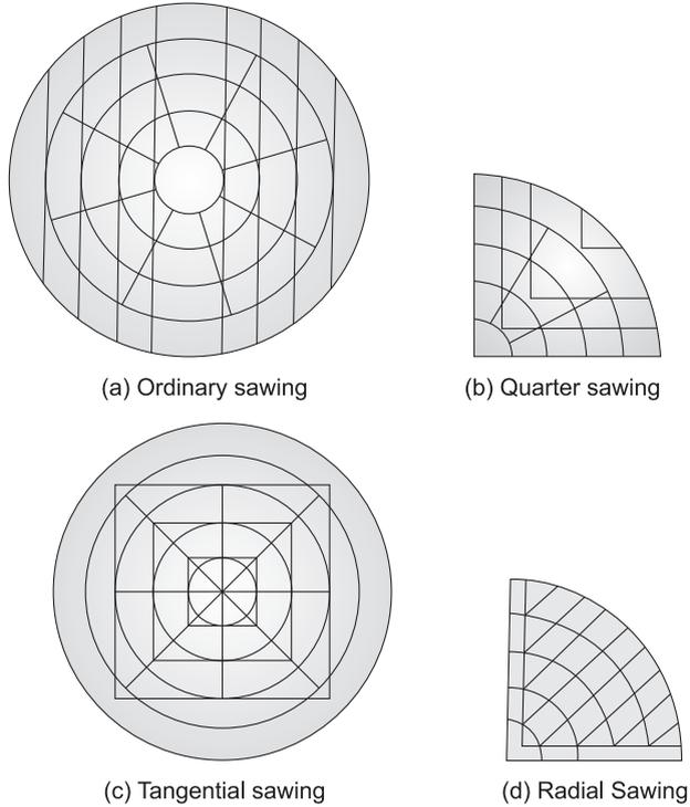
**Fig. 2.3** Methods of sawing
