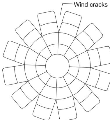
**Fig 2.9** Wind cracks
