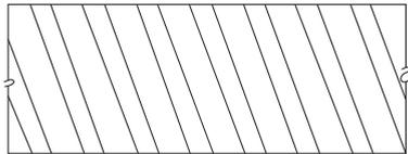
**Fig 2.8** Twisted fibre
