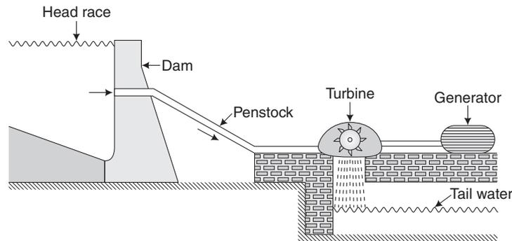
**Fig. 2.2** Layout of a hydrostation.
