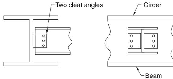
(f) Simple beam connections—beam to girder
