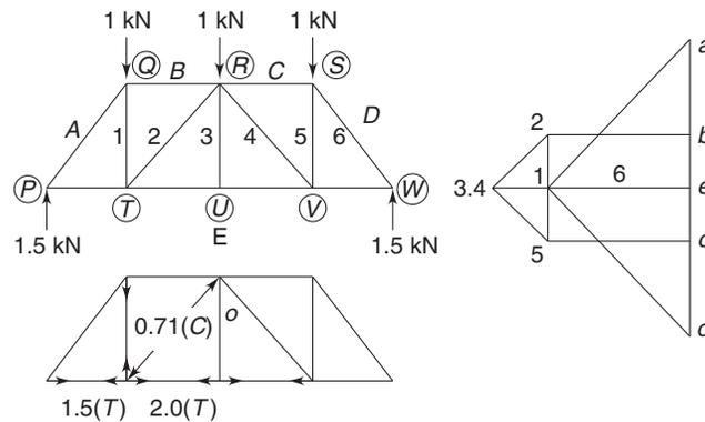
**Fig. 2.38** Vector diagram and force diagram
