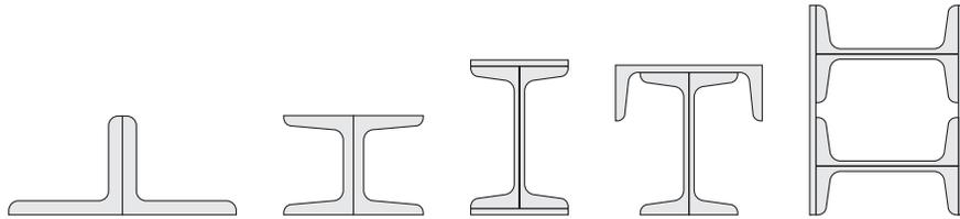
Fig. 2.2 Compound and built-up sections
