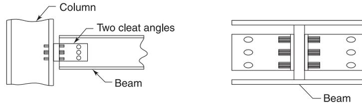
(j) Simple beam connections—beam to column
