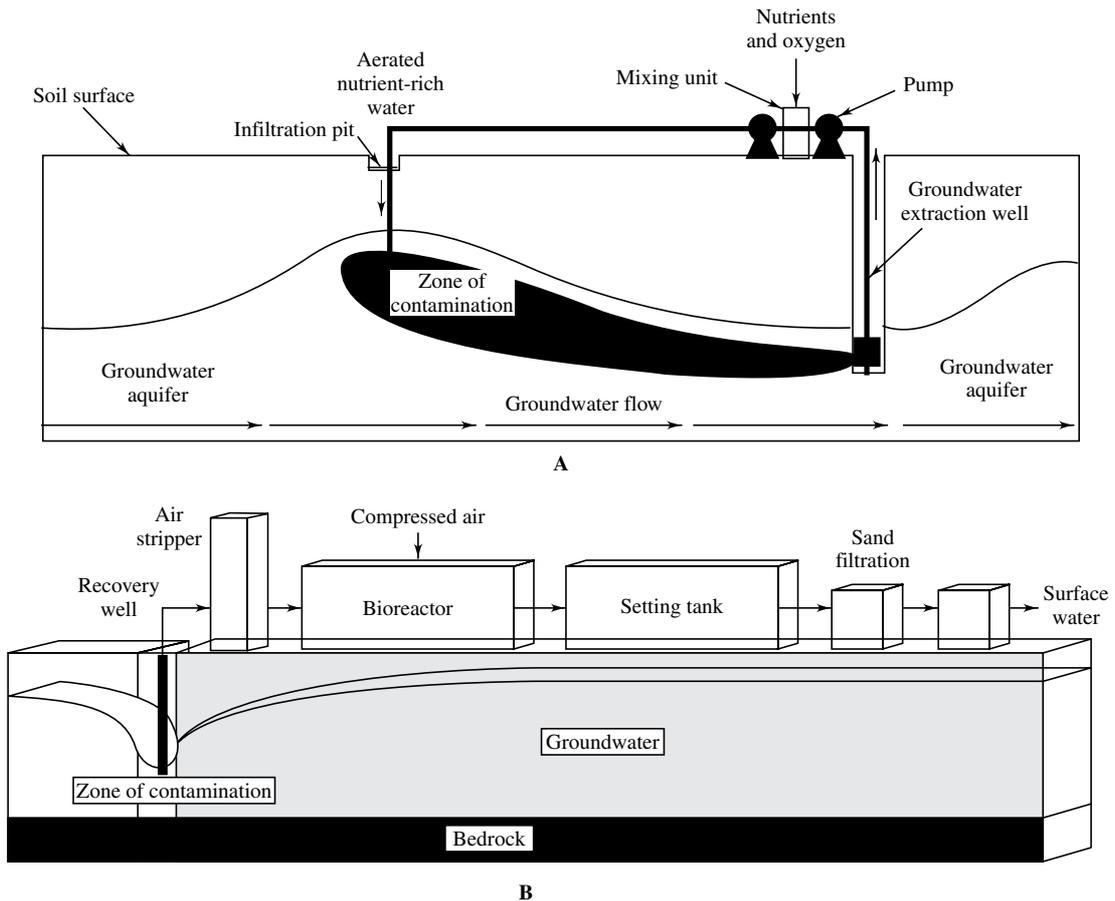
**Fig. 2.4** Bioremediation of subsurface contaminated soil and groundwater by (A) *in situ* and (B) *ex situ* bioremediation technology (Source: Atlas and Bartha, 1998).
