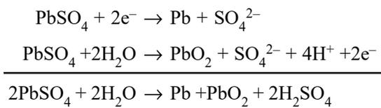
During charging, sulfuric acid is regenerated in the cell.
