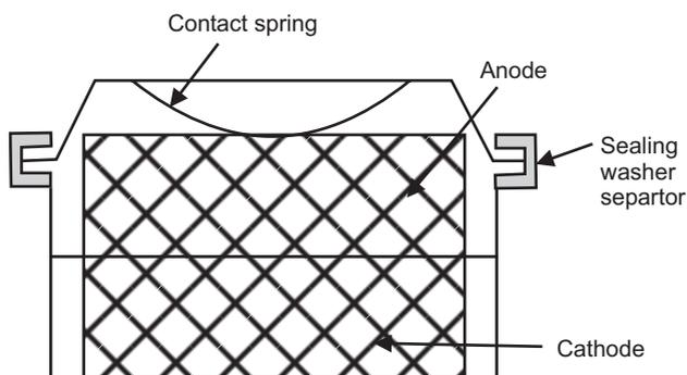
**Fig. 2.4.** Button type Ni-Cd cell
