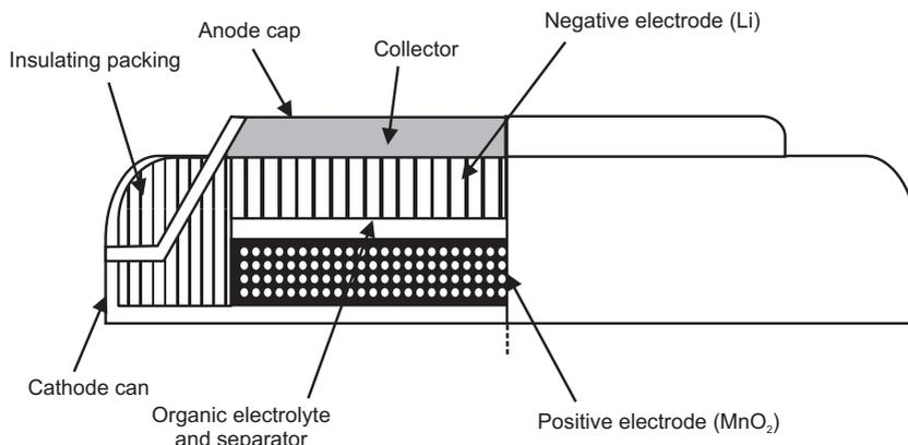
**Fig. 2.7.** Lithium- $\text{MnO}_2$  button cell
