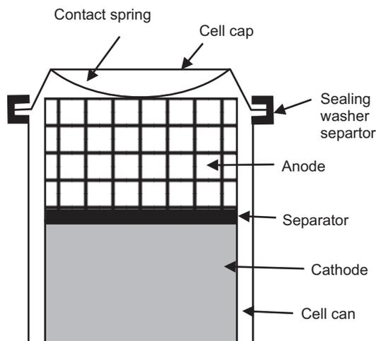
**Fig. 2.6.** Nickel-metal hydride button cell
