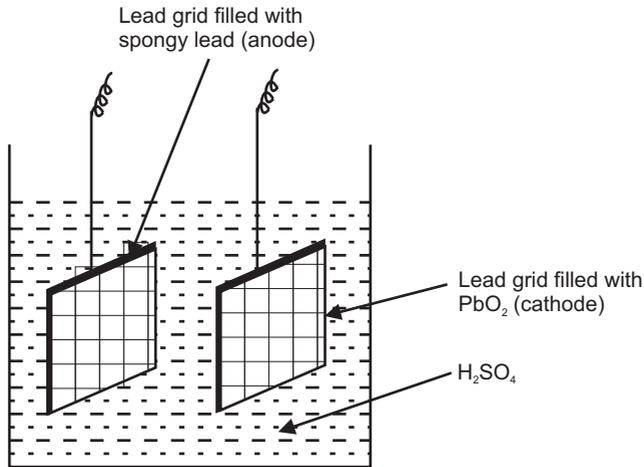
Fig. 2.3. Lead Storage Battery
