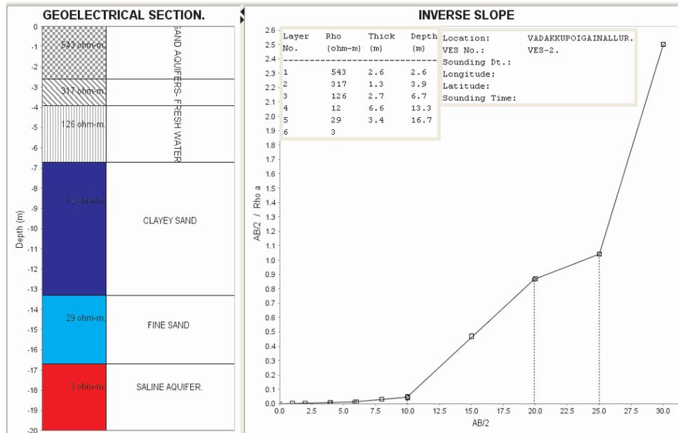
Fig. 4. Vadakkupoigainallur geoelectrical section – inverse slope.
