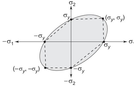
**Fig. 2.5** Distortion energy theory (Von-Mises criterion).
