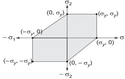
**Fig. 2.4.** Maximum shear stress criterion (Tresca's criterion)
