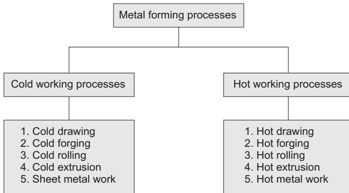
Fig. 2.6 Hot and cold working processes.
