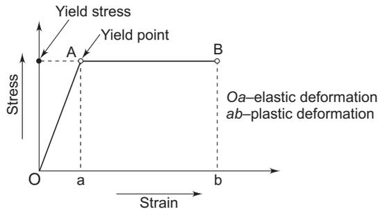
Fig. 2.1 Elastic and plastic deformation.
