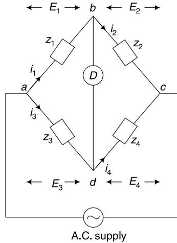
**Fig. 2.8** Basic ac bridge circuit
