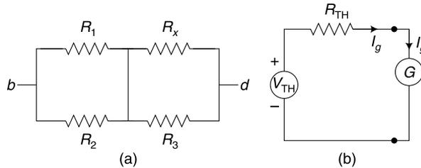
**Fig. 2.4** (a) Equivalent resistance ( $R_{TH}$ ) between  $b$  and  $d$ , (b) Thevenin equivalent circuit for Wheatstone bridge
