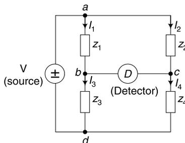
Fig. 2.1 General form of a bridge circuit
