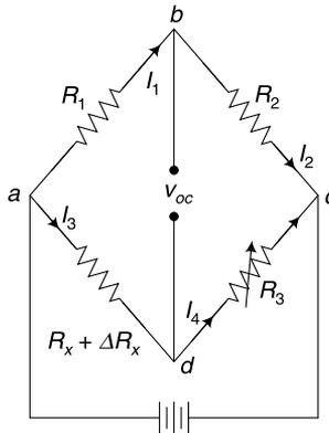
**Fig. 2.3** Wheatstone bridge under unbalance condition
