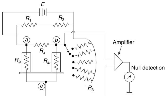
Fig. 2.7 High resistance measurement bridge
