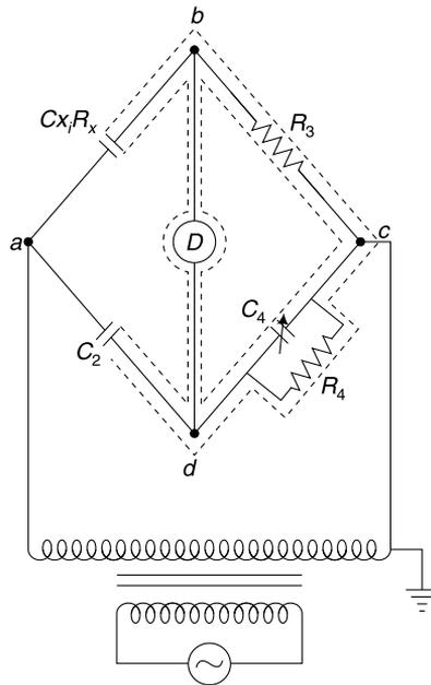
Fig 2.10 High voltage Schering bridge
