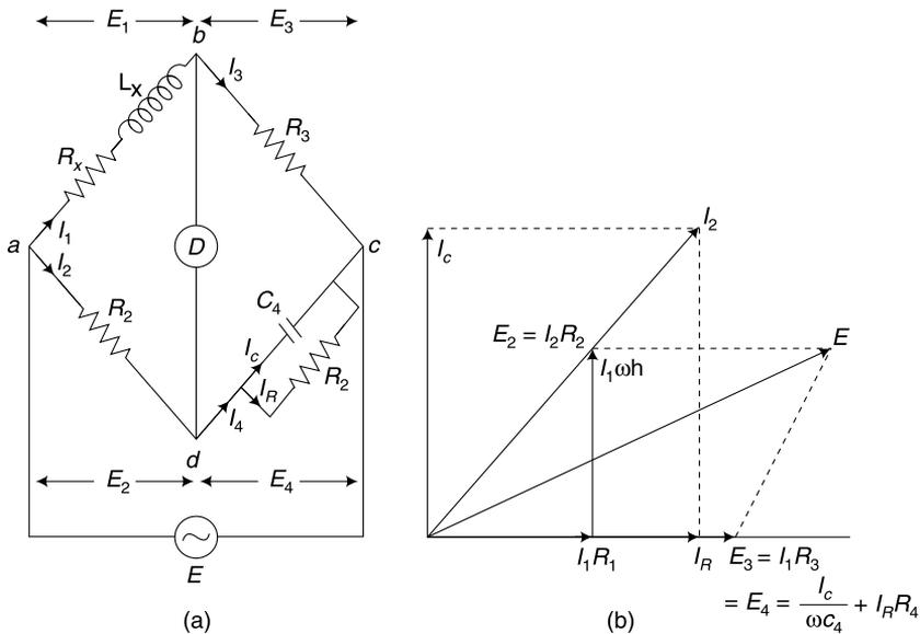
Fig. 2.13 (a) Maxwell inductance capacitance bridge
