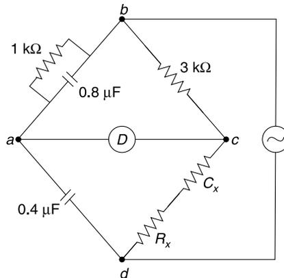
$$\begin{aligned} R_x &= \frac{C_4 R_3}{C_2} \\ &= \frac{3 \times 10^3 \times 0.8 \times 10^{-6}}{0.4 \times 10^{-6}} \\ &= 6 \text{ k}\Omega \end{aligned}$$
