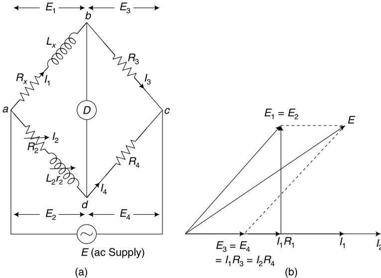
Fig. 2.12 (a) Maxwell inductance bridge (b) Phasor diagram
