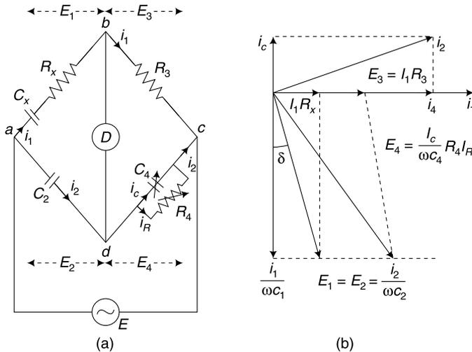
**Fig. 2.9** (a) Schering bridge for measurement of capacitance (b) Phasor diagram
