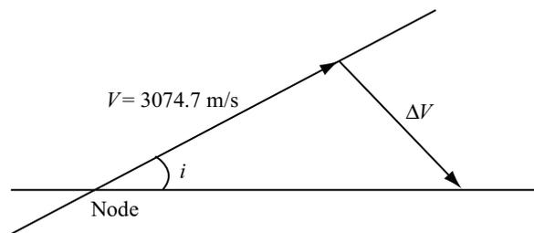
**Figure 2.5** Correction of the inclination of a synchronous orbit.
