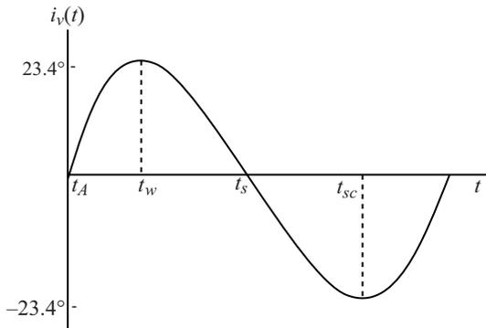
**Figure 2.9(a)** Sinusoidal variation of the earth's inclination angle.
