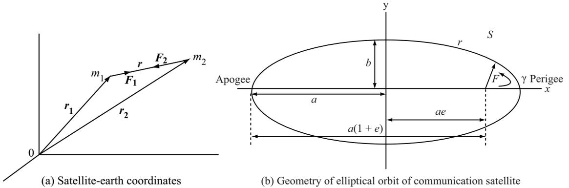
**Figure 2.1** Geometry of communication satellite.
