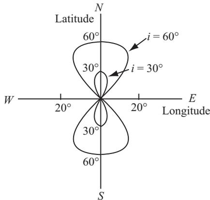
**Figure 2.4** Apparent movement of a satellite in an inclined and synchronous orbit with respect to the ascending node.
