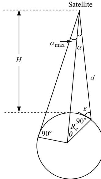
**Figure 2.8** Coverage angle and slant range.
