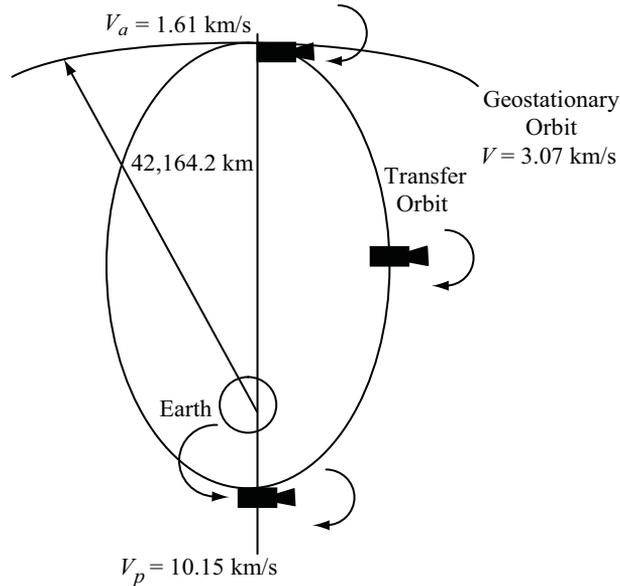
**Figure 2.13** Placement of a satellite in a geostationary orbit.
