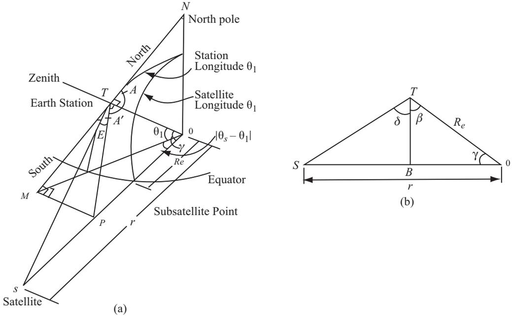
**Figure 2.7** Solar and sidereal days—triangle to calculate elevation.
