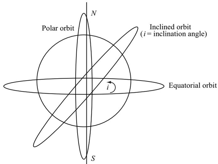
**Figure 2.2** Inclined orbits.
