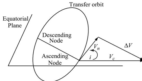
**Figure 2.14** Simultaneous orbit circularization and inclination correction.
