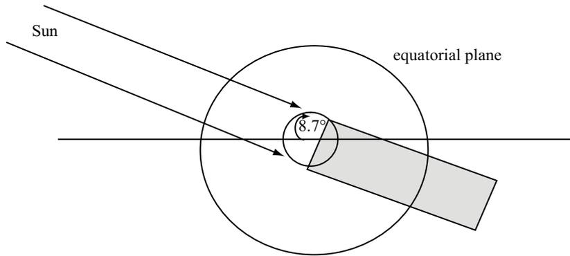
**Figure 2.11** Earth inclination at first day of eclipse before equinox.
