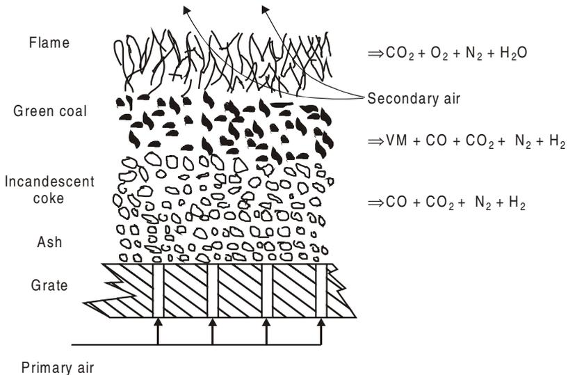
**Figure 2.15:** Principle of overfeed stoker.
