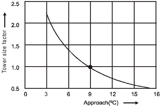
**Figure 2.59:** Effect of chosen approach on tower size.
