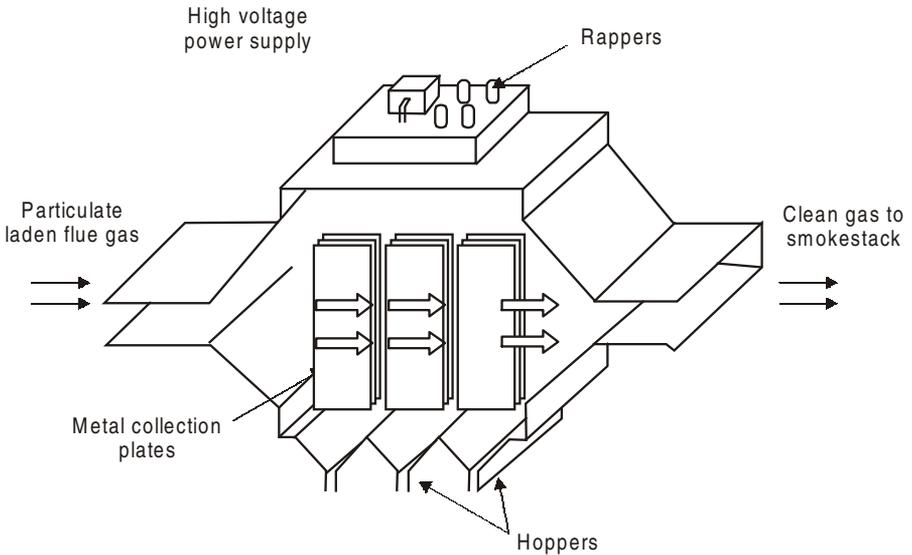
**Figure 2.27:** Side view of ESP schematic diagram.
