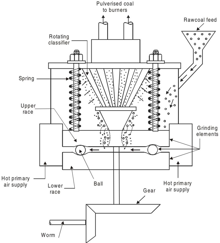
**Figure 2.9:** Ball and race mill.
