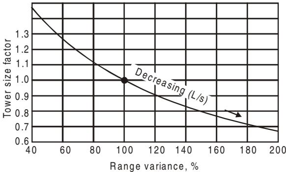
**Figure 2.58:** Effect of varying range of tower size.
