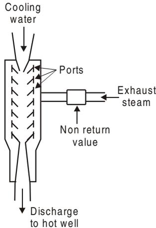
**Figure 2.37:** Ejector condenser.
