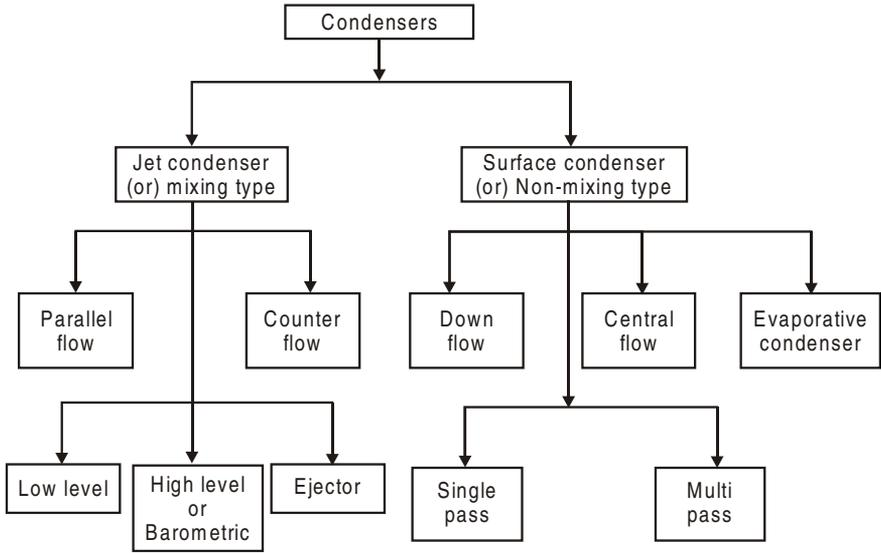
In jet condensers, there is direct contact between the cooling water and the steam which is to be condensed.
