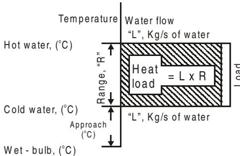
**Figure 2.56:** Parameters affecting tower size.
