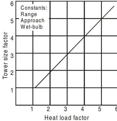
**Figure 2.57:** Effect of heat load on tower size.
