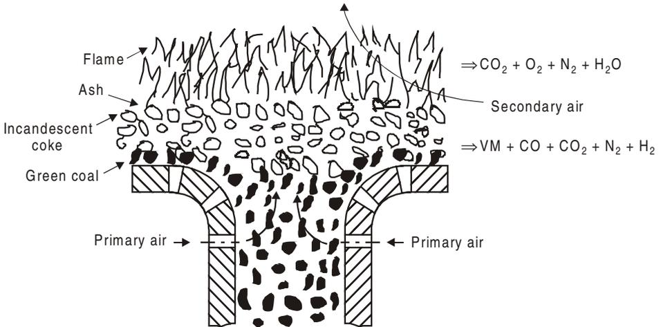
**Figure 2.16:** Underfeed supply of coal.
