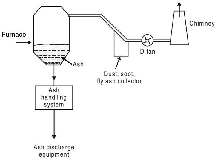
**Figure 2.21:** Ash handling equipment.
