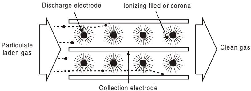
**Figure 2.26:** Top view of ESP schematic diagram.
