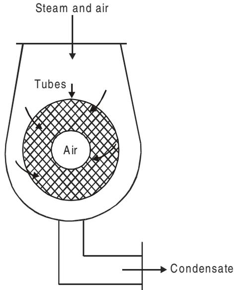
**Figure 2.40:** Central flow condenser.
