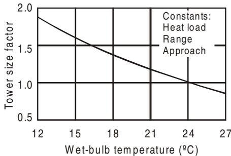
**Figure 2.60:** Effect of wet-bulb temperature on tower size.
