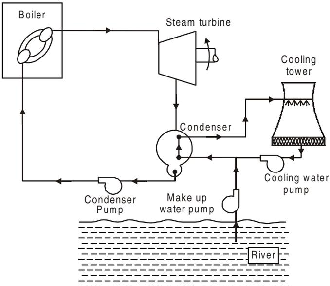
(b) Closed cycle condensing system
