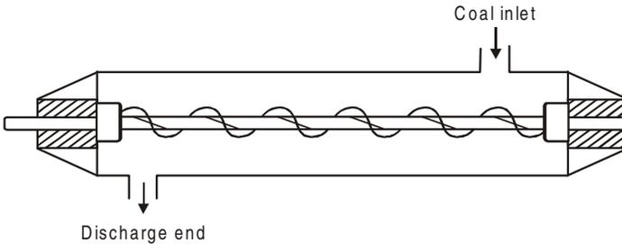
**Figure 2.3:** Screw conveyor.
