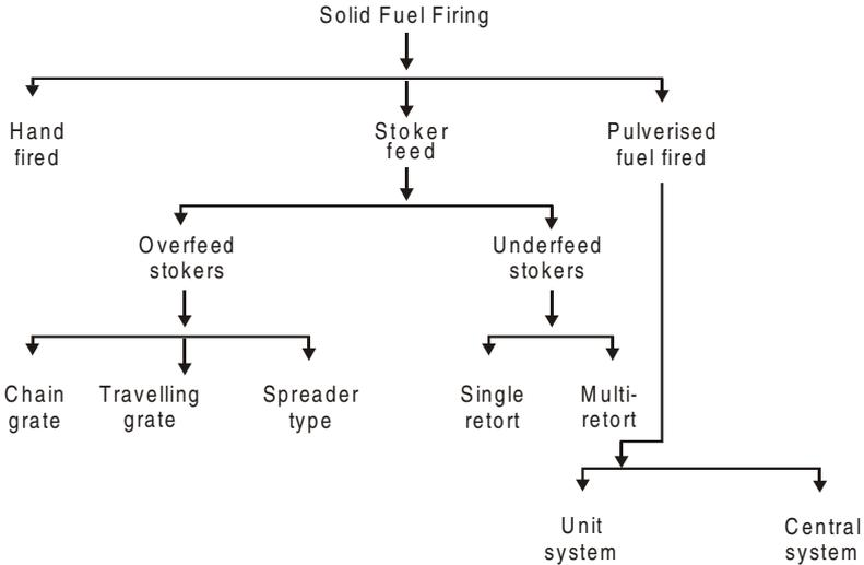
Common combustion equipment for steam boilers.
