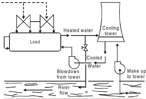
**Figure 2.43:** Closed-circuit system.
