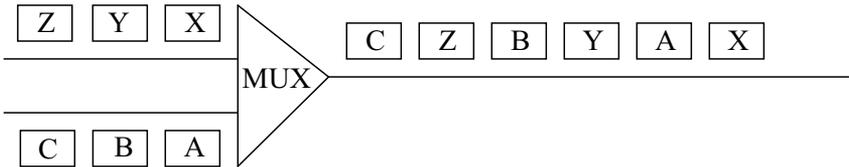
Fig. 2.28 Multiplexing using cells.
