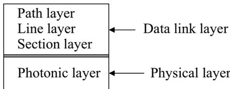
The photonic SONET layer describes the physical properties of the optical channels, receivers, multiplexing modes and other such things. The section layer transmits signals safely to the destination passing through different sections. The line layer passes the signals through different lines. The path layer is responsible for transmitting the signals from the source SONET to the destination one.
