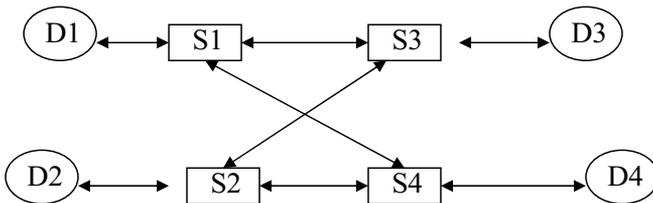
**Fig. 2.16** A typical switching network with four devices D1-D4 and for switches S1-S4.
