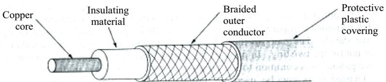
**Fig. 2.11** A coaxial cable.
