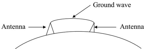
**Fig. 2.14** Movement of a ground wave in VLF, VF, and MF media.
