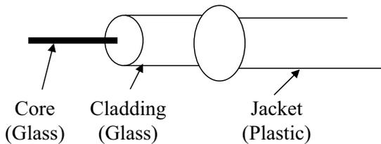
**Fig. 2.12** A fibre optic cable.
