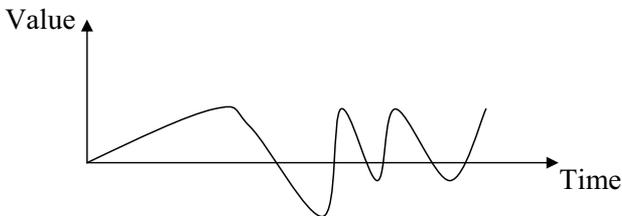
**Fig. 2.1** An analog signal.
