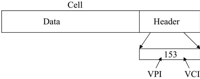
**Fig. 2.30** Virtual circuit identifier.
