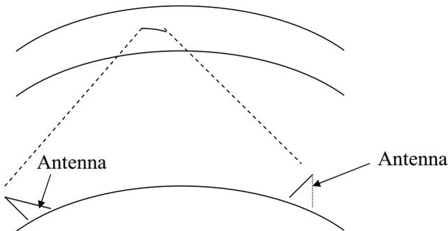
**Fig. 2.15** Refraction of radio wave to the earth from the ionosphere in HF mode.
