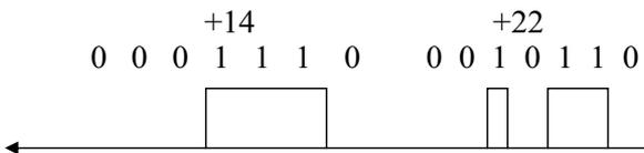
Fig. 2.25 Conversion of analog signals into digital codes.
