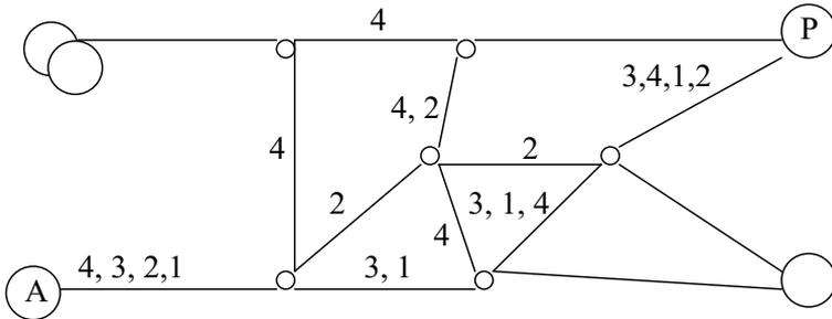
**Fig. 2.22** Datagram method of switching 4 packets.
