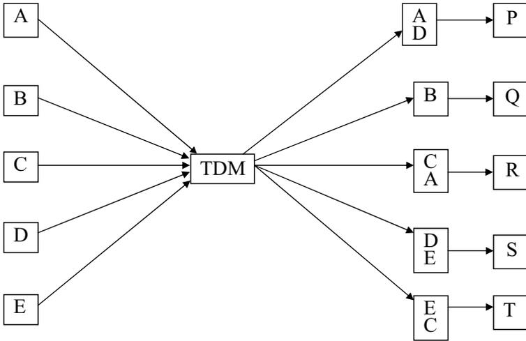
**Fig. 2.21** Time-division switching when no TSI is used.
