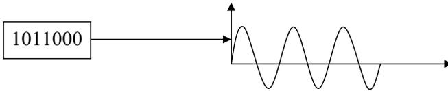
Fig. 2.26 Digital-to-analog encoding.
